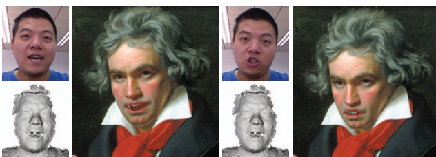
Fig. 11. Using a Kinect camera to track a user's facial expressions, which are then transferred to a still facial image, all in real time. This application allows a user to create an image avatar from a single facial image of another person.
